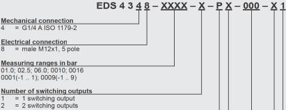
Output technology = programmable switching output
